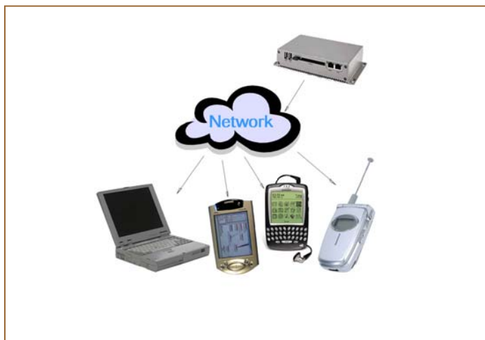
Figure 3: Example of the “ Push Strategy ”. The intelligent device gateway pushes data to the remote device.
