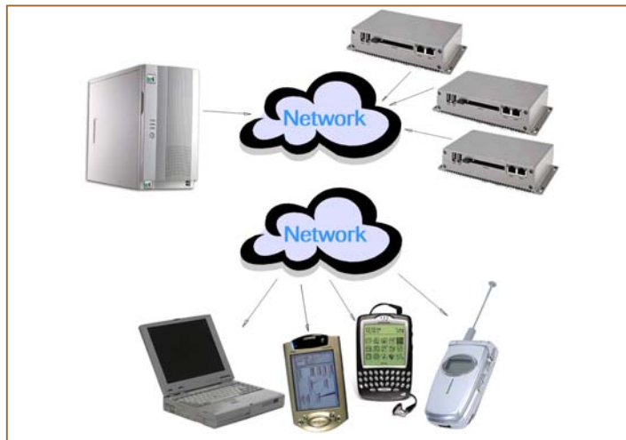
Figure 4—Example of the “Pull Strategy”. A server pulls data from the remote intelligent devices. The data is stored in a database from which it can be broadcast and made accessible via a variety of network protocols.
